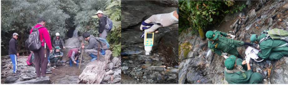
Figure 1: Water Discharge measurement... Figure 2: In-situ Chemical testing of water at Dingshinggar Figure 2: Macro-invertebrate survey to determine Water quality (biological quality testing)
